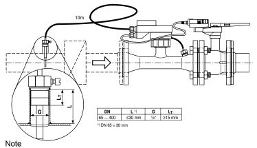
The cables between valve unit and temperature sensors may not be either shortened or lengthened.
