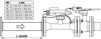
Installation of immersion sleeve and temperature sensor
