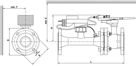
If Y <180 mm, then the extension of the hand crank must be dismantled as necessary.
