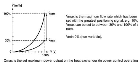
Vmax is the maximum flow rate which has been set with the greatest positioning signal, e.g. 10V. Vmax can be set to between 30% and 100% of V nom.
